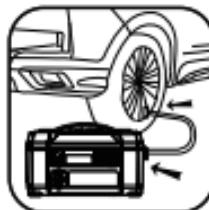
b. Wake up the product first by short press the LED light button or the power, then hold the pump button for 2 seconds to turn on the function.
